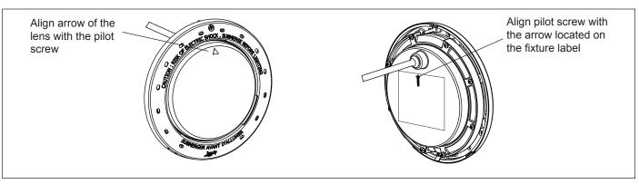
Figure 5. Alignment of the Lens, Face Ring, Housing and Clamps for Color Lights
