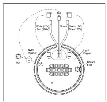
Figure 2. Small Light Engine (PCB) Replacement and Wiring
