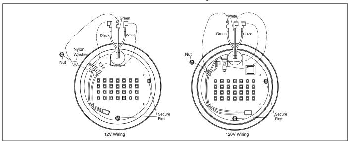
Figure 3. Large Light Engine (PCB) Replacement and Wiring
