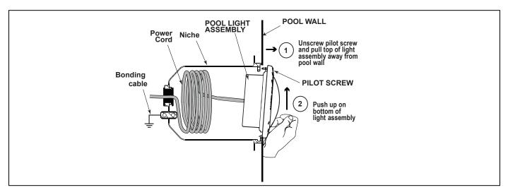
Figure 1. Removing the Jandy WaterColors Light Assembly for Light Engine Replacement
